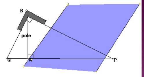
Joey is using a carpenter's square to find the distance across a river. He put the square on the top of a pole which is high enough to sight along a straight line from one of the legs of the carpenter's square across the river to point P. He then sights along the other leg of the carpenter's square in a straight line to a point Q. If QA is 2 feet, and BA (the pole) is 6 feet, find AP (the distance across the river).
